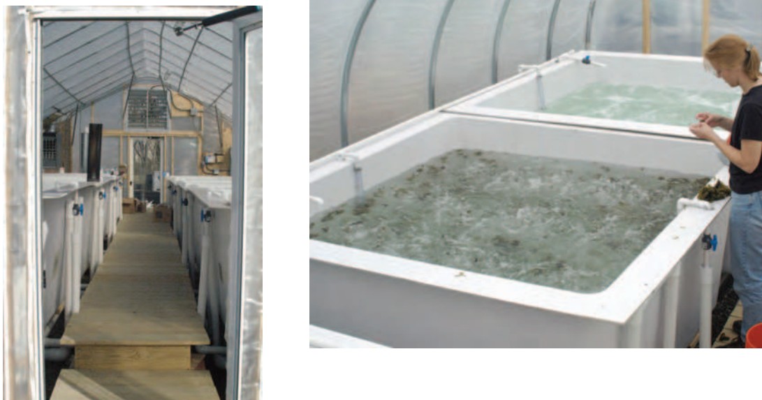
Figure 6.15. Greenhouse containing the experimental recirculating aquaculture system (left) and tank containing nori (right). Courtesy of Jennifer Day..
