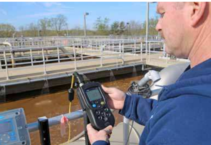
An operator at the H.L. Mooney Advanced Water Reclamation Facility (Woodbridge, Va.) validates the readings of a dissolved oxygen probe with handheld DO probe. Prince William County Service Authority
