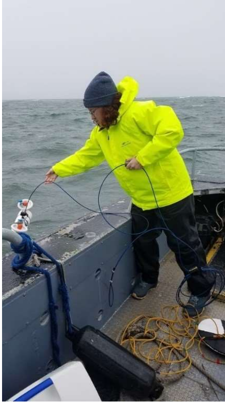
Cassidy Freudenberg, TOH C&W employee, using the Van Dorn water sampler. The sampler allows water to be collected at a known depth. (Photo courtesy of Dr. James Browne, ToH C&W.)
