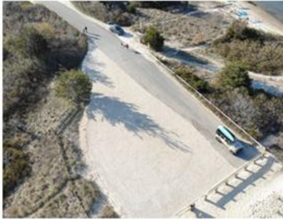
Louse Point Road Parking Area before and after. Impermeable asphalt was replaced with crushed quartz gravel to drain and filter stormwater. Photo Credit: Town of East Hampton
